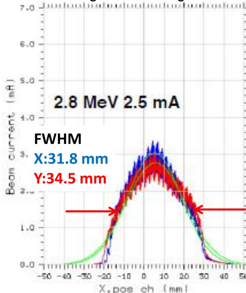
The profile was measured before setting the beam transport tube.
