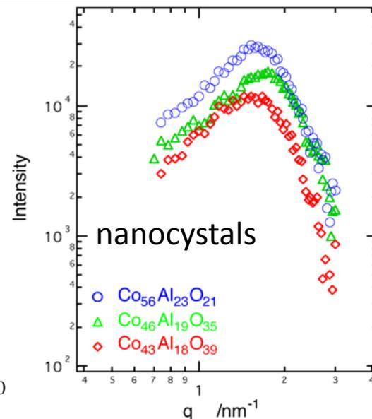
intermediate-Angle Neutron Scattering
